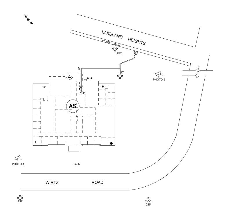
CONSTRUCTION- CLASS 3, NONCOMBUSTIBLE WALLS- STEEL FRAME FACED WITH 4 -INCH BRICK ROOF- METAL ON STEEL BAR JOIST WITH RUBBER MEMBRANE FLOOR- CONCRETE TOTAL AREA- 16,988 SQUARE FEET
